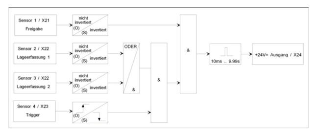
If the enable input is activated and the position sensors detect parts, the output for the set pulse time is activated with the (positive or negative) trigger edge.
