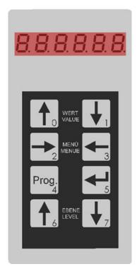
VALUE KEYS 0 and 1 MENU KEYS 2 and 3 PROGRAMMING KEY 4 SAVE KEY 5 LEVEL KEYS 6 and 7
